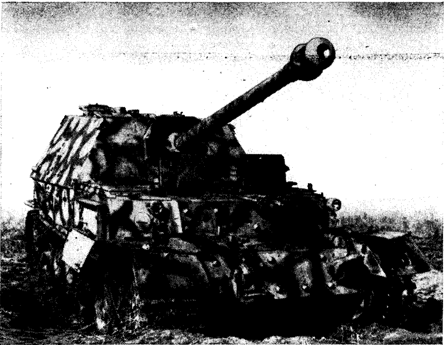
Figure 57.—88-mm self-propelled antitank gun ( Pz.Jäg. Tiger-P (Ferdinand) ). (Weight, 80 tons (approximately); maximum speed, 12 miles per hour; armament, 88-mm tank gun believed to be similar to the 8.8 cm Flak 41 .)
